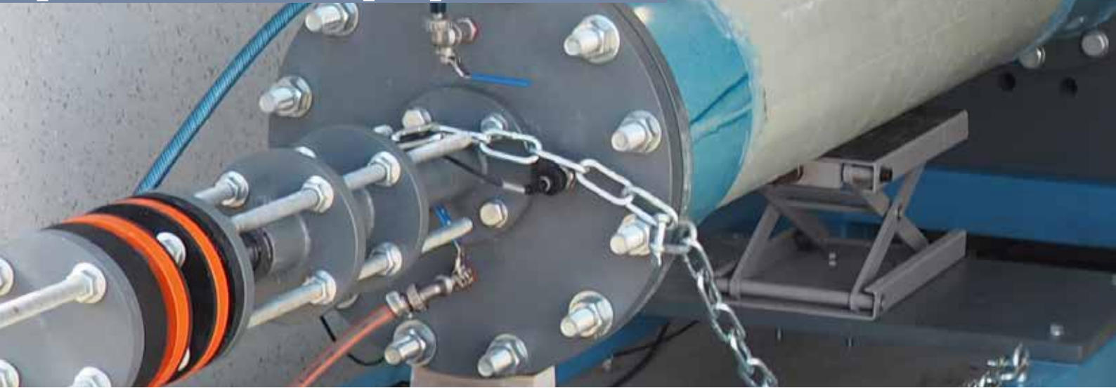
Dynamic-Load-Test facility of Siebert + Knipschild: dynamic analysis on pressure pipeline components
