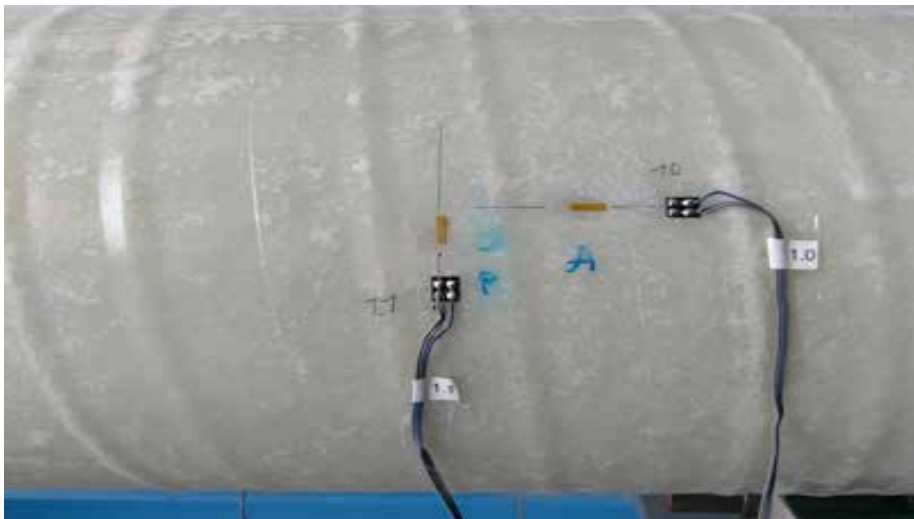
Strain gauges constantly capture changes in the material stretching in longitudinal and peripheral direction.
