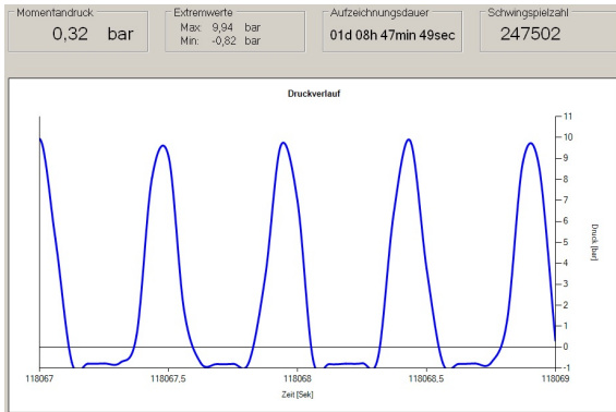
Pressure curve measurement
